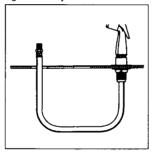
2 Insert spray hose down through hose guide and up through center hole in sink and putty plate.
